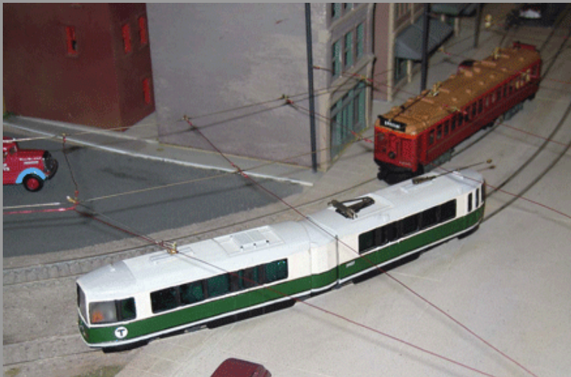
The 3402 ran all day Saturday without any problems. Current ground is by all four wheels of the power trucks only. The center truck contributes neither power or electrical grounding. The final floor will have provisions for couplers and headlight/taillights. Below is the 3402 negotiating an Hartel 9" radius curve.
